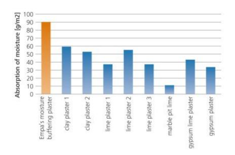
The moisture absorbing capacity of the novel Empa rendering system in comparison with competing products – the so-called "Nordtest."
