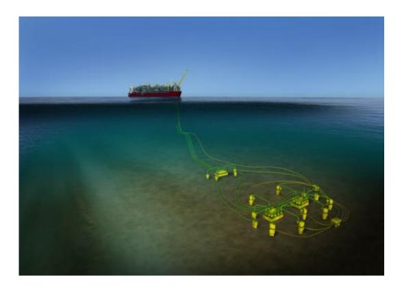
Mobile foundations provide an alternative solution to support seabed infrastructure. Credit: Shell
