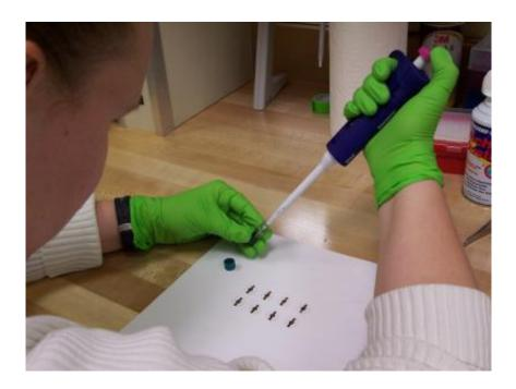
Small piezoelectric quartz crystals are the key to micro thermogavimetric analysis. Here, minute amounts of the test sample are deposited on the crystals. Credit: Kar/National Institute of Standards and Technology
