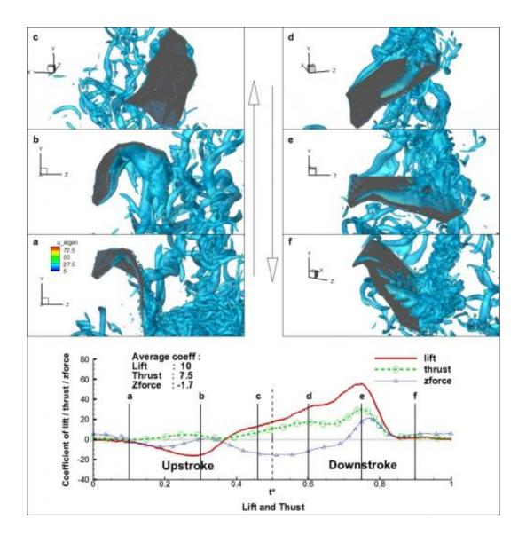
This is the time history of coherent vortex formation around the bat wing. Bottom plot shows lift and thrust coefficient variation for a flapping cycle over normalized time. Credit: D. Tafti/VT
