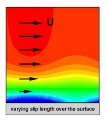
Understanding and successful modeling of flow over a surface characterized by spatially varying slip length, a phenomenon common in microfluidics, will help domain scientists and experimentalists generate future nano-device and lab-on-a-chip designs.
