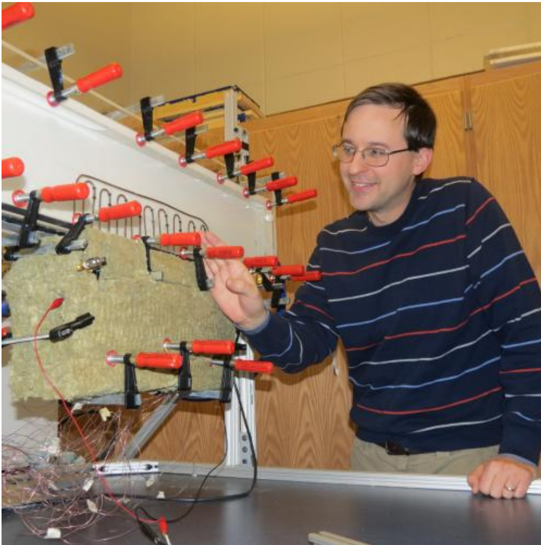
Assistant professor Gregory Michna explains the operation of the larger pulsating heat pipe model.
