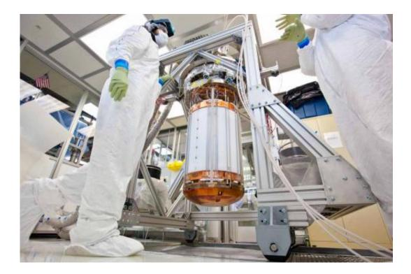
A new calibration technique fired neutrons directly into the Large Underground Xenon dark matter detector, increasing calibration accuracy by a factor of 10. Analysis based on the calibration confirms that if "low-mass" dark matter particles had passed through the detector during its initial run, Large Underground Xenon would have seen them. Credit: Matt Kapust/Sanford Underground Research Facility
