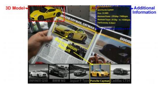
K-Glass recognizes the target object, which is a vehicle in this case, and then a 3D model of the vehicle is displayed on the top-left side with additional information on the top-right side. Credit: KAIST
