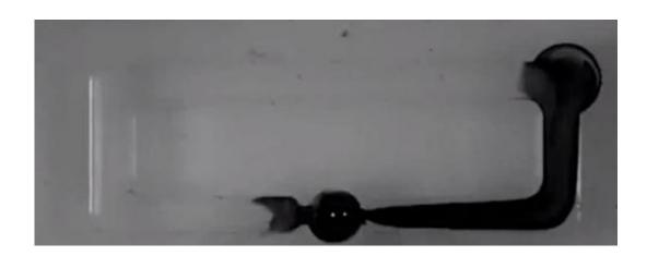
RMIT University researchers in Melbourne, Australia, have developed the world's first liquid metal enabled pump, a revolutionary new microscale device with no mechanical parts.
