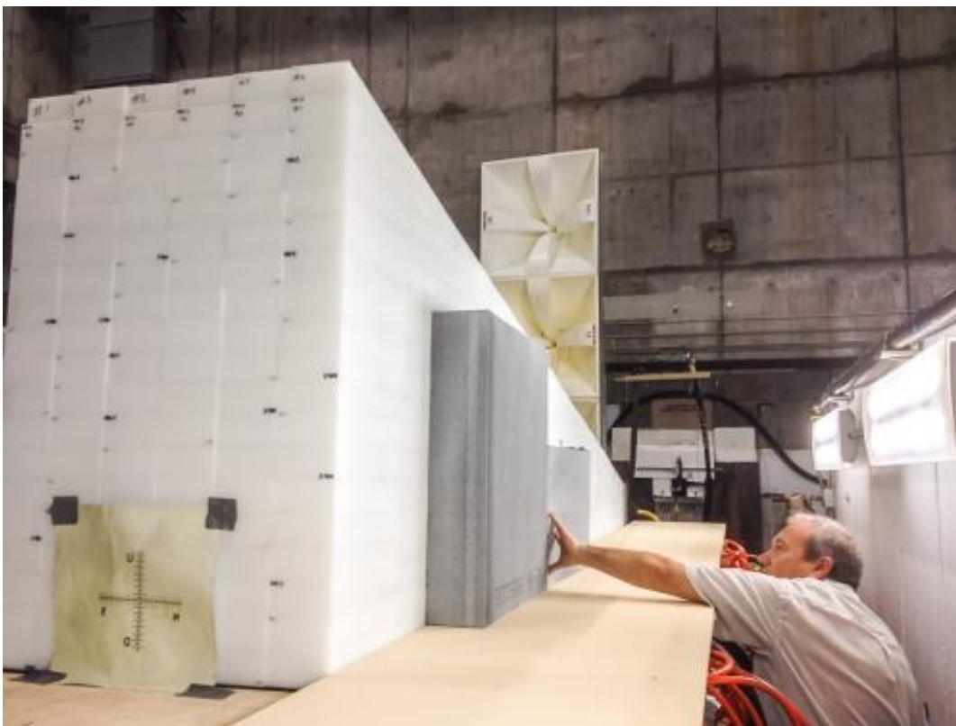
Principal investigator Konstantin Belov checks the placement of shielding around the plastic target - a stand-in for the Earth's atmosphere. Credit: Brian Rauch
