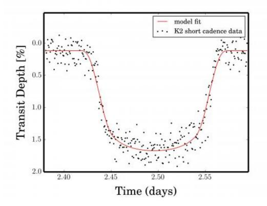
During a spacecraft operation performance test in Jan. 2014, one transit of the previous known exoplanet WASP-28b was captured. The data were obtained at 1 min intervals. The observation proves the repurposed spacecraft can still detect planets. Credit: NASA Ames/T. Barclay
