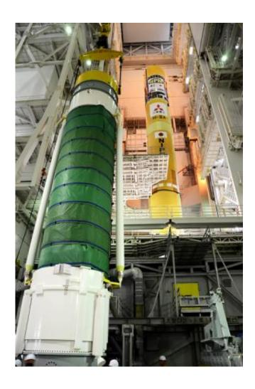
Attaching solid rocket boosters to GPM's launch vehicle, the HII-A No. 23. Credit: Courtesy Mitsubishi Heavy Industries
