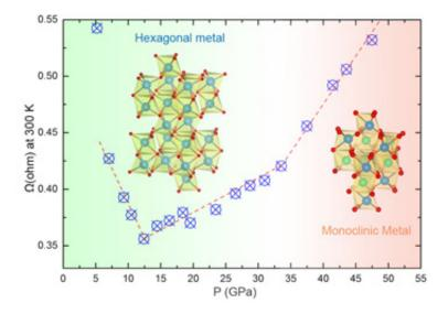
Electrical resistance as a function of pressure in V2O3. As pressure increases from 5 GPa, resistance decreases as expected. At 12.5 GPa the sharp increase in resistance is an unexpected result of electron-lattice interactions. At ~33 GPa, the material's corundum hexagonal structure changes to monoclinic, and resistance rises more sharply due to electron-electron interactions. Here the material is on the cusp of a metal-to-insulator transition.
