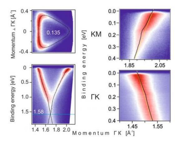
ARPES measurements of Calcium doped graphene. Left: the Fermi surface of graphene (top) and the Dirac cone (bottom). Right: The kink in the spectral function in the two crystallographic main directions. The scientists analysed the strength of the kink in order to estimate the superconducting critical temperature. Credit: A. Grüneis and A.V. Fedorov
