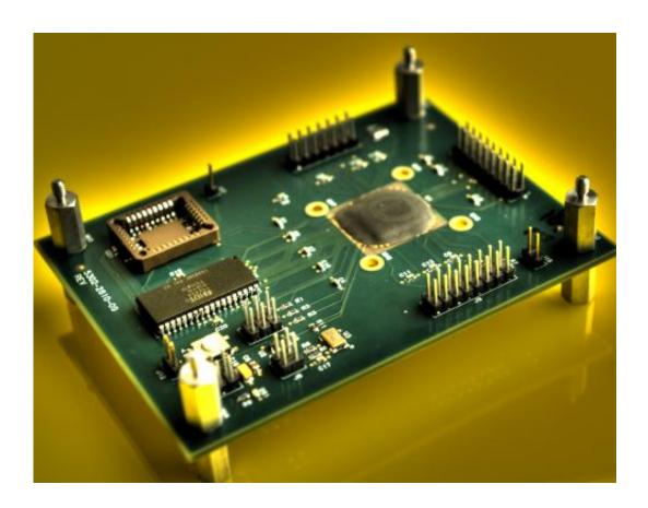
This is a close-up of the housekeeping chip that was bonded onto an electronics board as part of an investigation into the effectiveness of 3-D manufacturing for electronics applications. Credit: NASA
