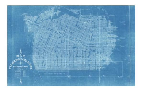
This map shows the underground workings of the Submarine Coal Mine, which operated from 1919-30 in Vigo County, Ind. Credit: Indiana Geological Survey
