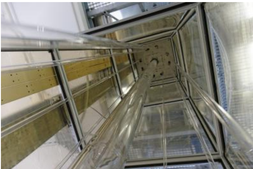
This is a laminar flow reactor from TROPOS. Credit: Photo: Tilo Arnhold/TROPOS
