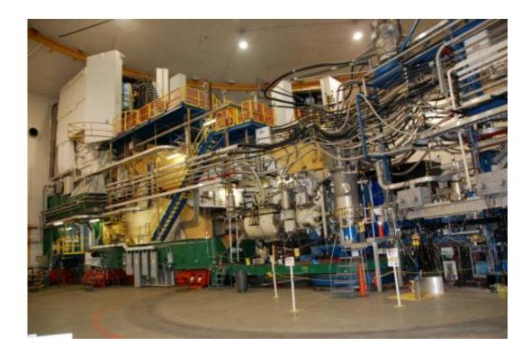
This is one of the four experimental halls at the US Department of Energy's Jefferson Lab. Hall A features two High Resolution Spectrometers (tall structures, each with white doors at the top) for nuclear and particle physics experiments. Credit: DOE's Jefferson Lab
