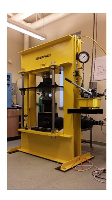
The rock deformation apparatus Skemer has built in his lab. The yellow frame is
