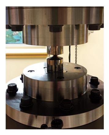
The business end of the machine. A pressure vessel supporting the rock sample is placed at the pinch point between tungsten carbide anvils at the center of this photograph. Credit: Skemer Lab
