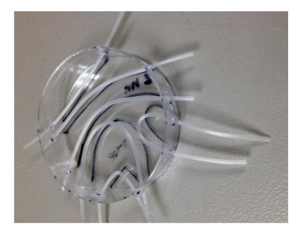
The mold for making a microfluidic device. Teflon tubes are inserted into a petri dish, then silicon is poured in. After the material hardens, engineers remove the disposable container and are left with an intact device. Credit: University of Washington
