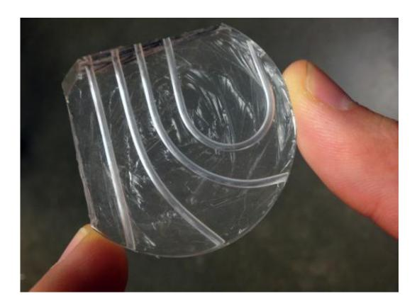
This prototype of a microfluidic device has both curved and straight channels for transporting tissue biopsies. The silicon material is lightweight, flexible and transparent. Credit: University of Washington
