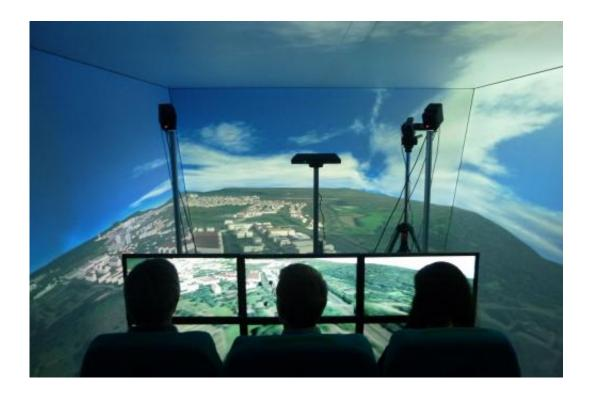
Participants are testing the set-up at Fraunhofer IAO: using Virtual Reality they get the impression of a transparent airplane cabin. Credit: Oliver Stefani, Fraunhofer IAO
