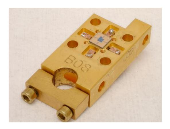
This NIST device, 1.5 by 3 centimeters in outer dimensions, is a prototype receiver for laser communications enabling much higher data rates than conventional systems. Superconducting detectors in the center of the small square chip register the timing and position of single particles of light. Credit: NIST
