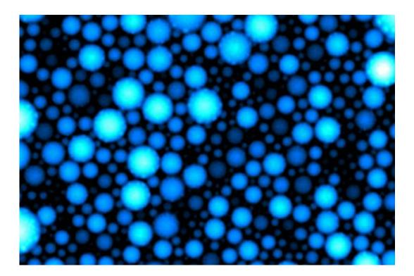
A complex oscillating reaction running in micro droplets as reaction vessels shows surprising variety in terms of period, amplitude and phase. With a fluorescent dye integrated into one of the reaction steps, the team of scientists from Technische Universitaet Muenchen and the University of California (Pasadena and Riverside) were able to investigate the reactions. Credit: Maximilian Weitz / Technische Universitaet Muenchen
