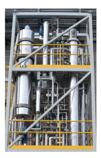
At this facility, AVA Biochem produces 5-(hydroxymethyl)furfural from biomass. The compound can serve as a precursor for various materials. Credit: AVA Biochem
