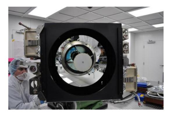
Roughly the size of a refrigerator, CATS will use the same two laser wavelengths on NASA's CALIPSO mission, 1064 and 532 nanometers, and it will incorporate a third laser wavelength--355 nanometers. This will provide more detailed information about the particles in Earth's atmosphere. Credit: NASA
