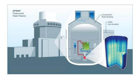
CASL is developing and applying new modeling and simulation technology (Virtual Environment for Reactor Applications Core Simulator or VERA-CS) to resolve and predict the detailed neutron distribution of the power-generation reactor core residing in reactor vessels. Credit: Westinghouse.
