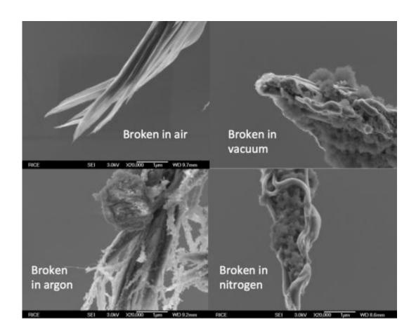
Scanning electron microscope images show typical carbon nanotube fibers created at Rice University and broken into two by high-current-induced Joule heating. Rice researchers broke the fibers in different conditions – air, argon, nitrogen and a vacuum – to see how well they handled high current. The fibers proved overall to be better at carrying electrical current than copper cables of the same mass. Credit: Kono Lab/Rice University
