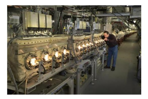
Stochastic cooling "kickers" generate electric fields to nudge ions in RHIC's gold beams back into tightly packed bunches. This system of squeezing and cooling beams has produced dramatic increases in collision rates—and the data coming out of RHIC. Credit: BNL
