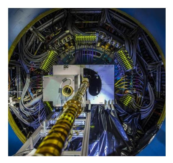
The central portion of the Heavy Flavor Tracker (HFT) being installed at RHIC's STAR detector. The HFT will track particles made of "charm" and "beauty" quarks, rare varieties (or "flavors") that are more massive than the lighter "up" and "down" quarks that make up ordinary matter. Credit: BNL
