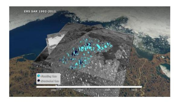
Floating ice (light blue) and grounded ice (dark blue) in lakes of Alaska's North Slope near Barrow, as seen by ESA's ERS-2 satellite in 2011. Credit: Planetary Visions / University of Waterloo, Canada / ESA
