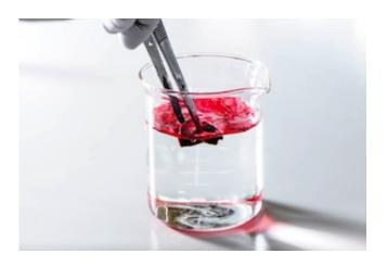
Here the sponge-like aerogel soaks up only the red-dyed diesel fuel in a beaker of water.
