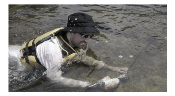
Tom Gleeson in Ontario's Tay River with a temperature-conductivity probe to detect groundwater coming out of bedrock fractures. Credit: Tom Gleeson
