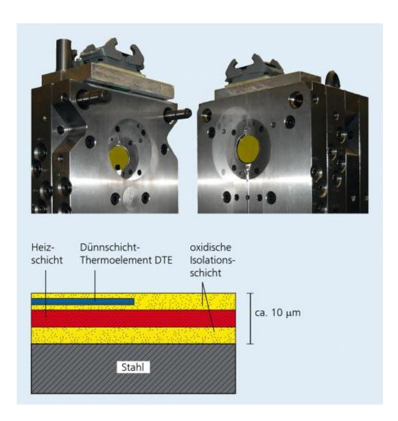
More cost-efficient plastic components with improved surface quality: This injection-molding tool is equipped with thin-film tempering coatings (round area on each half of the opened tool). Credit: Fraunhofer IWM
