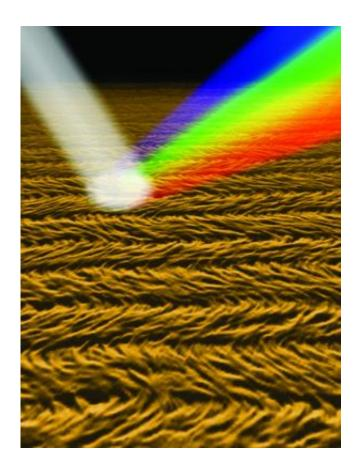
Bioinspired phage-based colourimetric sensors, termed Phage litmus, are composed of hierarchical bundles like the collagen fibres in turkey skins. Application of target molecules (chemical stimuli) causes colour shifts due to structural changes, such as bundle spacing (d1 and d¬2), and coherent scattering. Through the colour change analysis, we can identify target molecules in a selective and sensitive manner. Credit: Seung-Wuk Lee & Jin-Woo Oh
