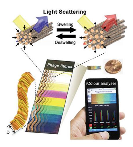
Bio-inspired sensors are made from bacteriophages that mimic the collagen fibers in turkey skin. When exposed to target chemicals, the collagen-like bundles expand or contract, generating different colors. The researchers also created a mobile app to be used with camera phones to help analyze the sensor's color bands. Credit: Seung-Wuk Lee Laboratory
