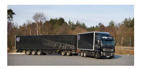
Trucks that are between 18.76 and 25.25 metres long are more ecofriendly than the shorter "European" trucks. Research at Chalmers University of Technology now also shows that these vehicles are at least as safe as shorter trucks in traffic. Testing with even longer trucks is currently ongoing in Sweden.
