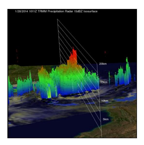
TRMM satellite flew above a tropical low (91S) in the Mozambique Channel on Jan. 28, 2014, at 1011 UTC and this 3-D view using TRMM PR data shows that some towering storms near the center of the low were reaching heights of above 16km (about 9.9 miles). Credit: NASA/SSAI, Hal Pierce
