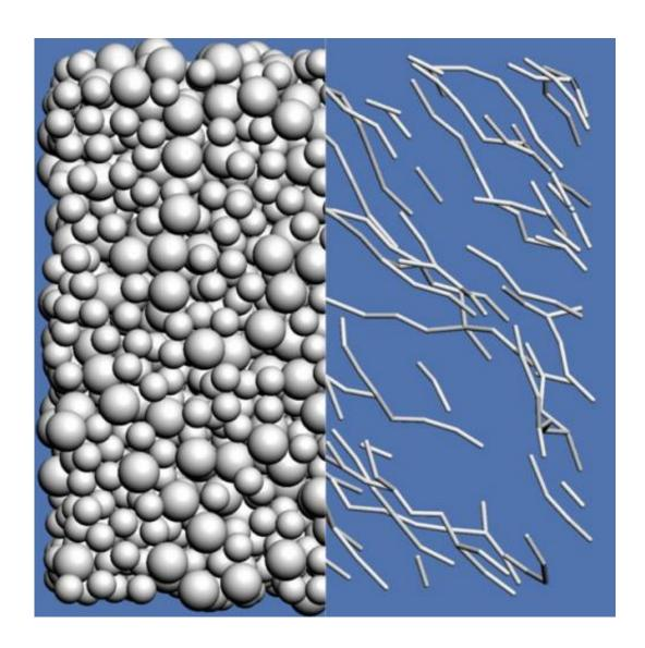
Sheared suspension of spheres occupying 52 percent of a volume, alongside images of "force chains;" i.e., the paths connecting spheres as they come into contact with their neighbors. The top image shows the spheres sheared before the transition to discontinuous sheared thickened. Credit: Benjamin Levich Institute,
