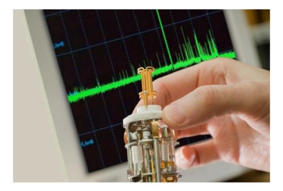
An international team of researchers has greatly expanded the potential for NMR analysis apparatus. They have made it possible to measure all the signals of a substance with a single, newly developed miniature antenna, while in current equipment several – very expensive – antennas are needed to do so. Moreover, only a few nanolitres of a substance are needed to conduct measurements. Previously, half a millilitre was
