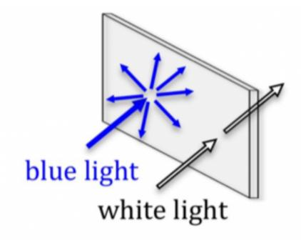
The basic principle for the new transparent projection screen: nanoparticles that interact with a single color (in this case blue) are incorporated into a transparent material. The result is a material that lets most of the ambient light go through and therefore appears transparent; however, by using a laser projector that sends a blue light beam of the specific color that is scattered by the embedded nanoparticles, one can obtain a high-resolution projected image. Credit: Chia Wei Hsu
