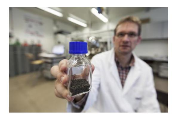
Zeolites bind the water produced during methanation of hydrogen, thereby increasing the methane yield from the new process. Credit: Empa
