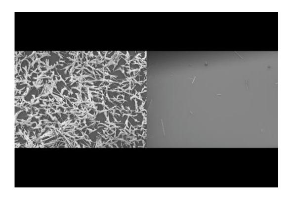
A comparison between an untreated smooth surface (left) and lubricantimpregnated surface (right), after having gypsum-rich water boiled away from it in the lab. The treated surface shows significantly less scale deposition.
