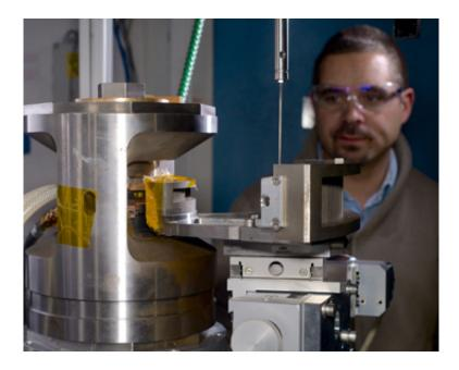
The experimental set-up at the ESRF beamline. The Paris-Edinburgh press is to the left ; the magma rock sample is compressed in its centre to pressures of up to 36.000 atmospheres, and then heated by a resistor to up to 1700 degrees Celsius. The slits on the right filter the X-ray beam reaching the detector. Credit: ESRF/Blascha Faust
