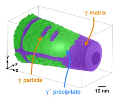
The  $\gamma$  matrix (purple) can be seen surrounding the cuboidal  $\gamma$  precipitates (green). Only a few nanometre-sized  $\gamma$  platelets can be seen in the  $\gamma$  precipitates. Atom probe tomography allows a site specific analysis of the structure at the atomic scale and reveals the chemical composition in measurements of individual areas. Credit: HZB
