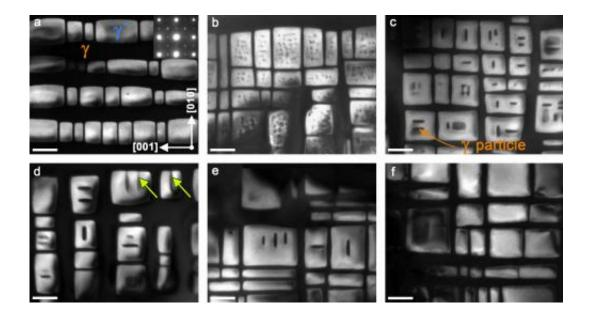
The TEM micrographs reveal how small spheres (dark areas) initially form through heating (b), coalesce into platelets (c), until they split the  $\gamma$  precipitates (d-f). Scale bar widths: 100 nm. Credit: HZB
