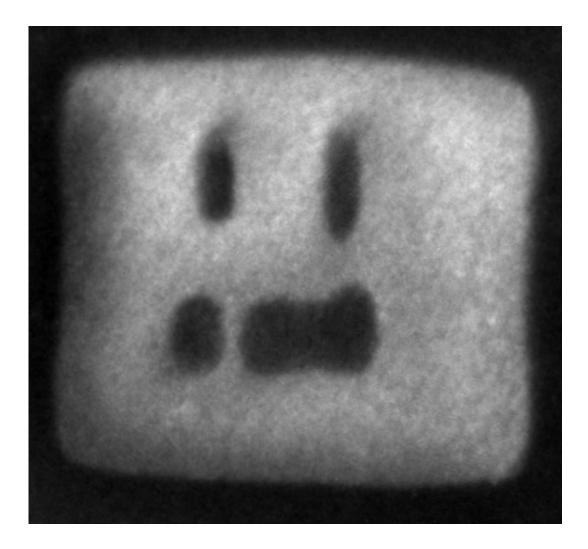
This image shows a about 100 nm large  $\gamma$  precipitate (light area) surrounded by the  $\gamma$  matrix (dark area). Plate-like  $\gamma$  particles (dark areas) can be seen within the  $\gamma$  precipitate. Credit: HZB
