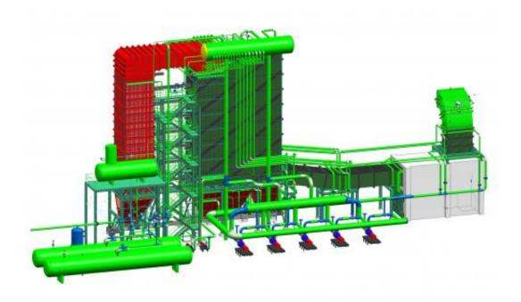
A new solution from Siemens takes advantage of hot flue gases from arc furnaces to generate steam. This steam can then be used for other steel mill processes or for generating electricity. In the past, flue gases were usually not utilized, so the energy they carried was lost. The system consists of steam boilers, pipes, water tanks, and pumps and can be directly integrated into the existing flue gas cooling system. Theoretically, the system could entirely replace conventional cooling.
