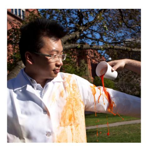
Former postdoctoral fellow Tak-Sing Wong demonstrates the difference between SLIPS-coated and untreated fabrics. The SLIPS-coated sleeves of the lab coat repel wine, tomato juice, eggs, and more; the untreated body of the jacket does not. Credit: Eliza Grinnell, SEAS Communications
