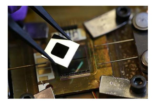
A nanophotonic solar thermophotovoltaic device as viewed from the perspective of the incoming sunlight. Reflective mirrors boost the intensity of the light reaching the carbon nanotube absorber array (center), enabling the device to reach high temperatures and record-setting efficiencies. Credit: FELICE FRANKEL
