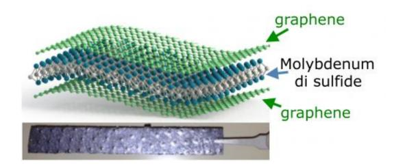
A Kansas State University engineer has made a breakthrough in rechargeable battery applications. The bottom image shows a self-standing molybdenum disulfide/graphene composite paper electrode and the top image highlights its layered structure. Credit: Gurpreet Singh, Kansas State University
