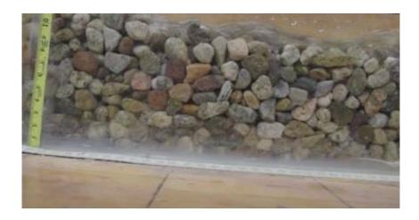
Artificial river in the earth surface dynamics lab at caltech built to model the behavior of steep channels. Credit: Jeff Prancevic
