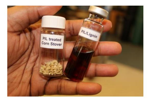
The new process dissolves lignin into low-cost protic ionic liquids, leaving cellulose behind as a solid. Credit: Ezinne Achivinu, North Carolina State University
