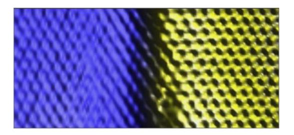
ORNL and UT researchers have invented a method to merge different 2-dimensional materials into a seamless layer. This colorized scanning tunneling microscope image shows a single-atom sheet composed of graphene (seen in blue) combined with hexagonal boron nitride (seen in yellow). Credit: ORNL
