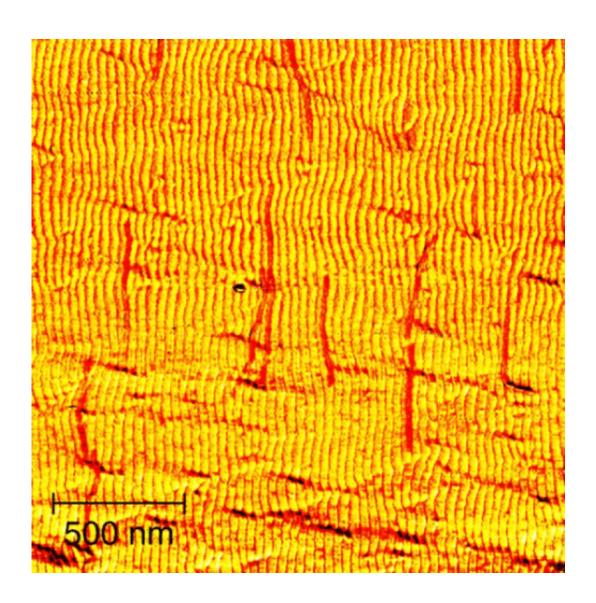
What looks like sand dunes is actually smaller than a single grain of sand. Thanks to electrostatic surface interactions, DNA nanotubes (shown here in red) align along the prefabricated nanopattern on a silicon surface. Credit: Helmholtz-Zentrum Dresden-Rossendorf
